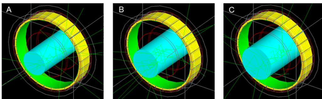
**Figure 4.** The representative figures for the (A) 50, (B) 70 and (C) 90 kg phantom using the Monte Carlo simulation. The radius of phantom was determined based on relationship between abdominal circumference and body weight.
