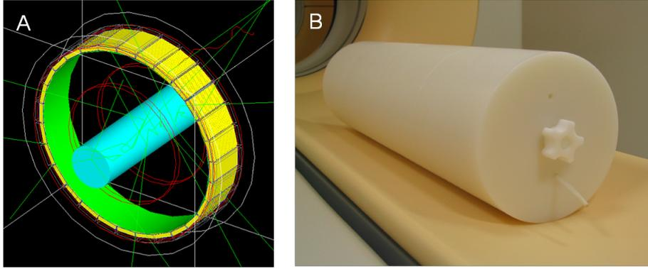
**Figure 1.** (A) Schematic of the Monte Carlo simulation for the measurement of scatter fraction and (B) scatter fraction phantom according to the NEMA NU2-2007 guidelines.
